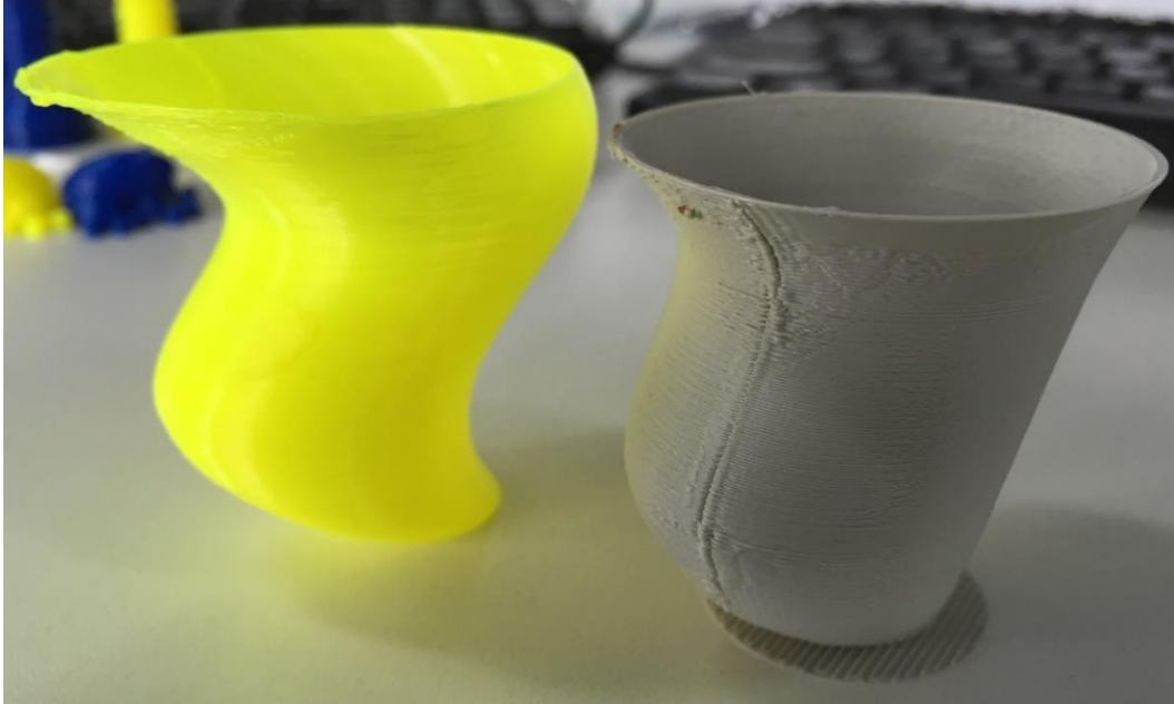
Figure: A visible seam on the grey object. The yellow was printed with the 'random' option.
