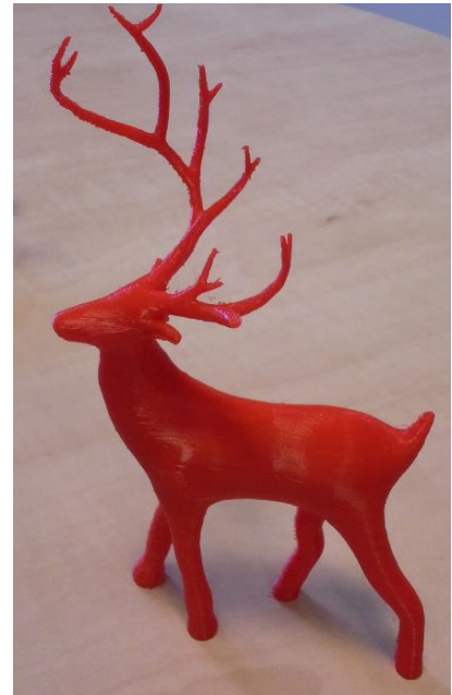
The deer pictured is printed at 25mm/s, but the antler was printed much slower, automatically.
